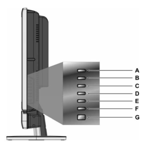
Α Input Select the Input source. Confirm OSD menu selection. В **Volume Up** Increase volume or adjust a highlighted increasingly control while in OSD menu. C **Volume Down** Decrease volume or adjust a highlighted control decreasingly while in OSD menu. D CH Up Channel up/ Scroll up. **CH Down** Е Channel down/ Scroll down. MENU F Turn OSD menu ON/OFF. Power G Turn the power ON/OFF.
